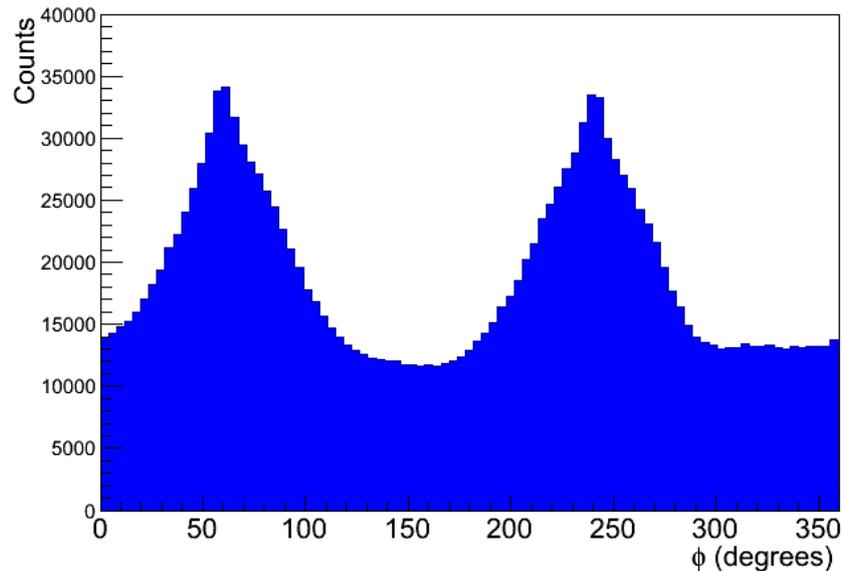
Fig.9: Azimuthal angle distribution of the muons. Peaks around 60 and 240 degrees are due to the rectangular geometry of the chambers and their orientation w.r.t. North.
