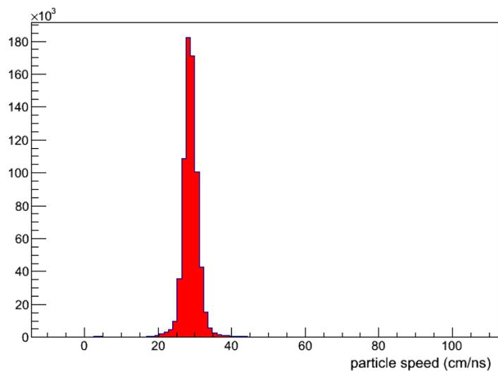
Fig.7: Distribution of the ratio between track length and time-of-flight of single tracks in the MRPC chambers.
