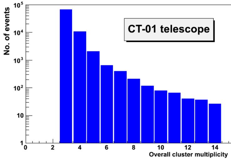
Fig.4: Overall cluster multiplicity in the MRPC chambers of the EEE CT-01 telescope.
