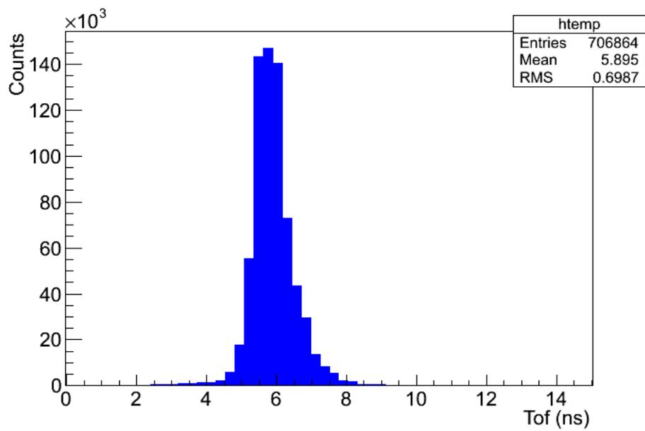
Fig.6: Time-of-flight distribution of single tracks in the MRPC chambers.
