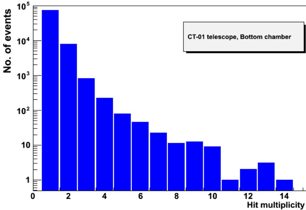
Fig.1: Hit multiplicity in one of the MRPC chambers of the EEE CT-01 telescope.
