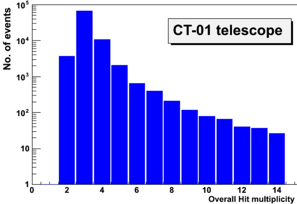
Fig.2: Overall hit multiplicity in the three MRPC chambers of the EEE CT-01 telescope.
